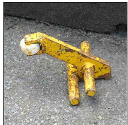
A sidearm for Pandrol track. Make sure you have the correct type
