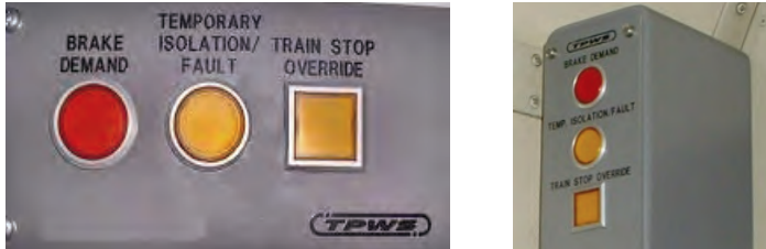
Examples of standard TPWS control panels
