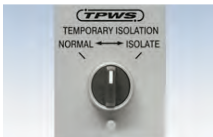
TPWS temporary isolation switch
